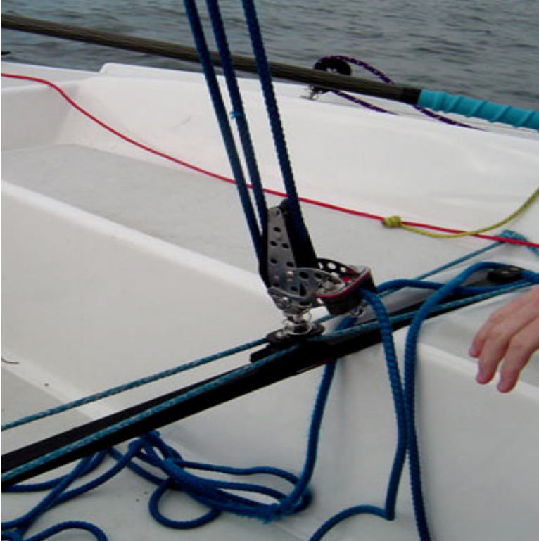
Position the traveler just below the weather seat in light winds to help keep the boom close to centerline.
