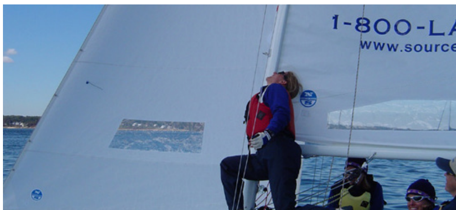
Sight the sag in the mast by sighting up the back of the mast when sailing upwind.
